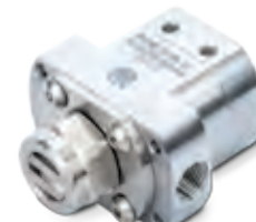
AA10000AUH-104215 Front port for liquid recirculation Typical flow range: 0.0017 - 0.47 gpm (0.006 - 1.8 lpm) Stainless steel, Viton or EPDM seals, PPS and PEEK Up to 15,000 cycles per min
