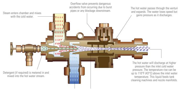
The cold water instantly condenses the hot steam and creates a vacuum. The cold water absorbs the heat and velocity from the steam and a high-speed stream of hot water is produced.
