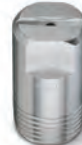
U 1" to 2" male conn. Flow rates of 40 gpm and greater at 40 psi (151 lpm and greater at 2.8 bar)
