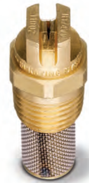
H-VV and H-VVL 1/8" to 1/4" male conn. Flow rates below 1 gpm at 40 psi (3.8 lpm at 2.8 bar) H-VVL includes integral strainer
