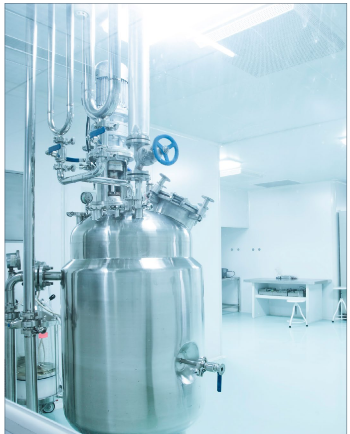
A typical vessel used for bioprocessing.
