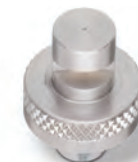
QSTK Spray Tip Miniature version Flow rates below 1 gpm at 40 psi (3.9 lpm at 2.8 bar) Use with seal and QJJS body
